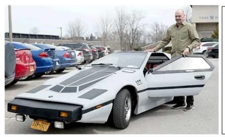
This is an Urba Centurion, a strange looking home built car that is really economical. It achieved better than 250 mpg at a recent event held at Watkins Glen and cruises at 70 Mph! It is registered for, and can be seen at the concours. A Kubota 3 cyl diesel engine powers the car that was built from plans first published by Mechanix Illustrated in February 1982. Plans are still available from
